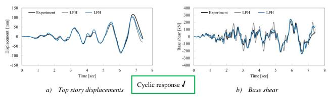
Figure 3. Comparison of the experimental results and numerical prediction of the RC bare frame for models LFH & LPH.
