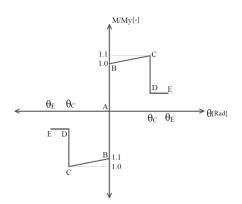
a) Moment plastic hinge model for beams
