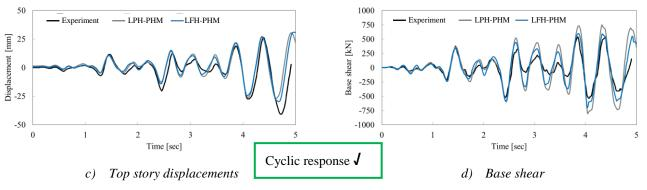
Figure 4. Experimental vs. numerical results of the RC frame with infill walls for model: LFH-PHM & LPH-PHM.
